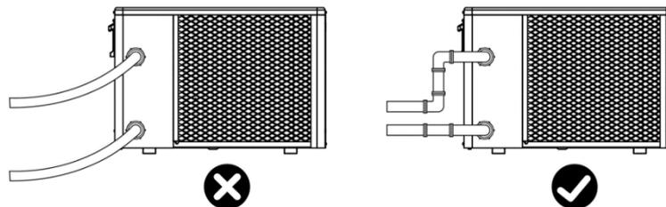
2. To ensure heating efficiency, the length of the piping between the pool and the heat pump should be less than 30ft.
