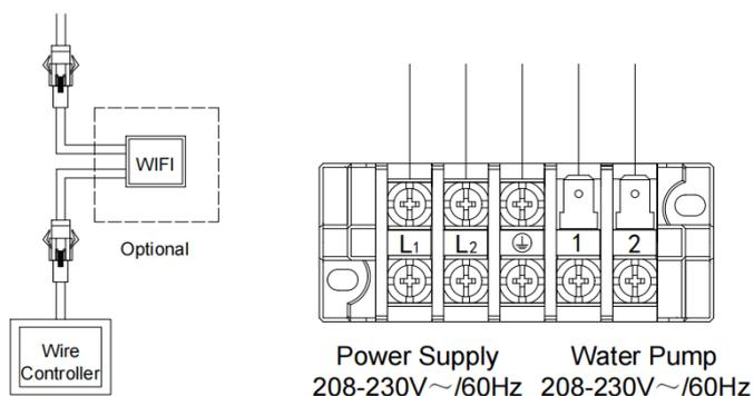
Note: If the water pump wattage is more than 800 Watts, Do Not Connect it to the terminal block inside the heat pump. Use an external contactor, and a separate breaker
