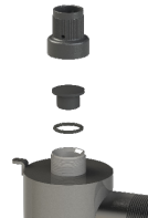
Pressure Test Cap Installation
